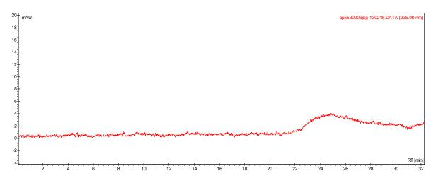
Analysis Method: Varian Prostar system with 1 ml/min DCM flow across four Phenogel 5u columns (Agilent). Detection via UV/Vis, calibrated against polystyrene standards
